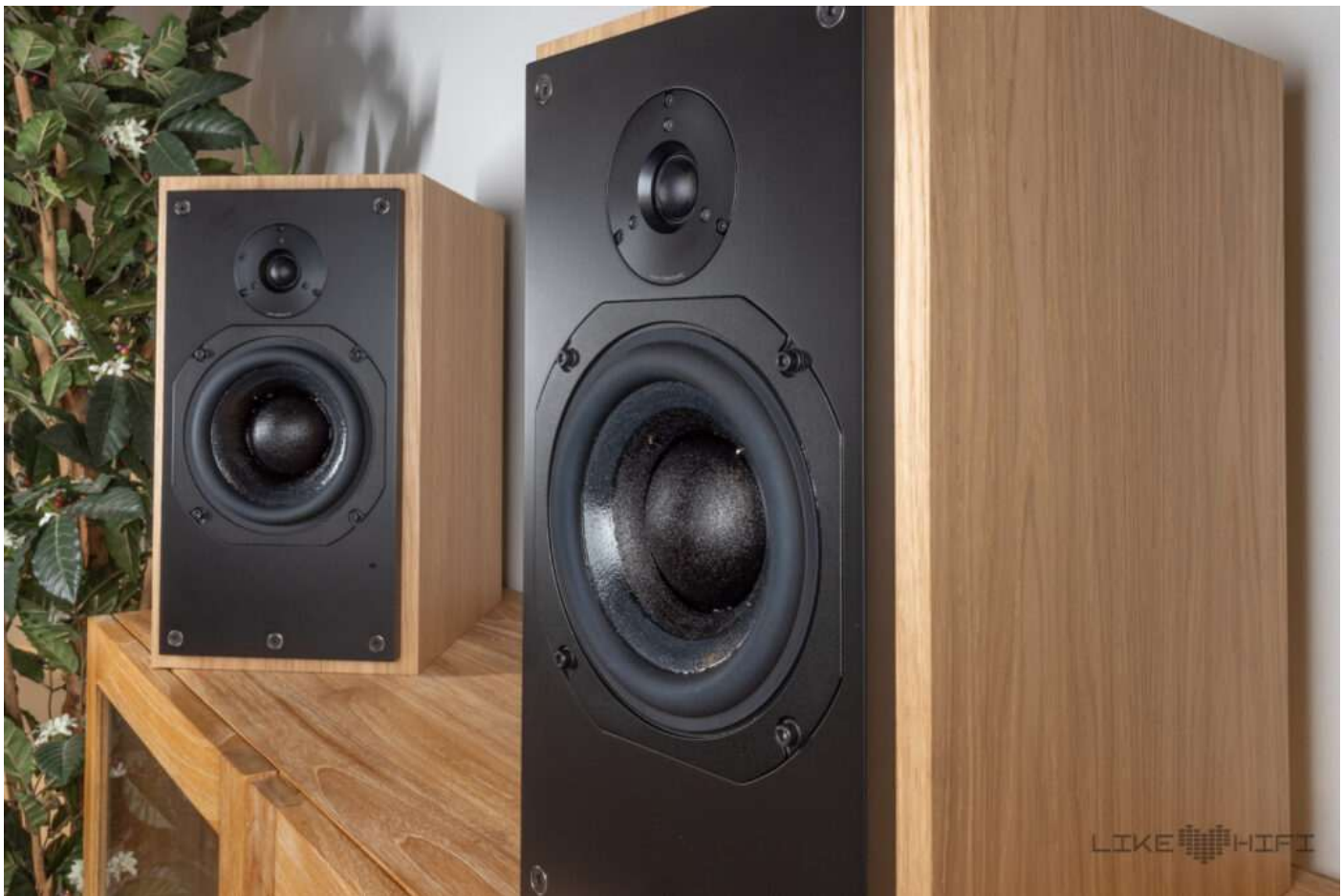
The 2-way system with a closed cabinet is a classic design that proves its worth once again. (Image: Auerbach Verlag)
